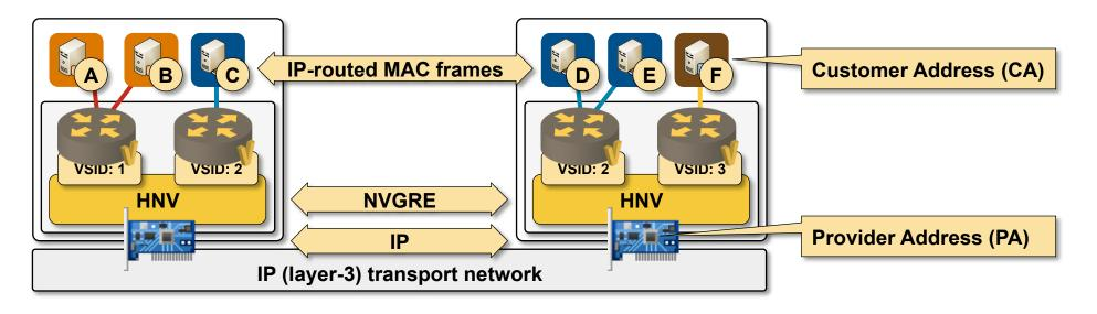
Full layer-3 switch in the hypervisor (distributed routing functionality)
