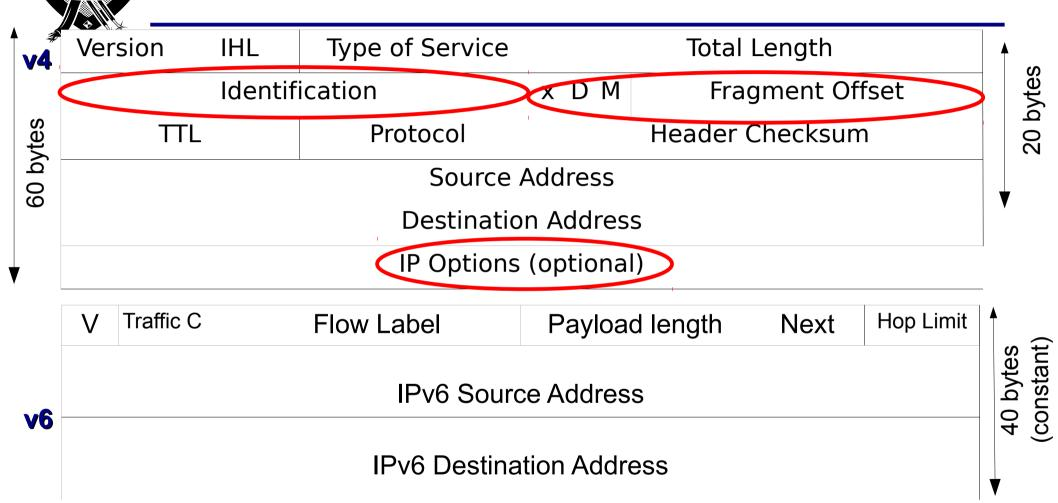
**IPv6 Extension headers** have been introduced to support any extra functionality, if required.
